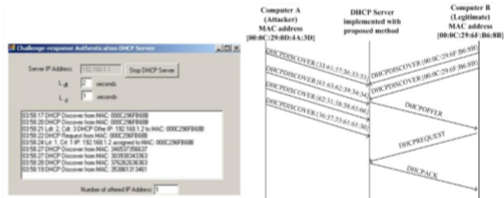
Fig. 3: The set-up scenario with malicious and legitimate DHCP client
