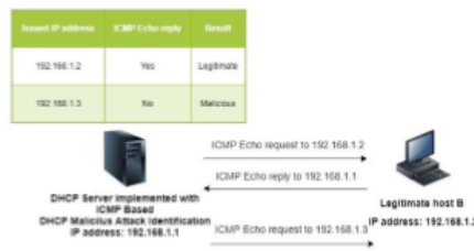
Fig. 2. The DHCP malicious request identification based on ICMP[5]
