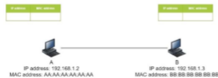
Fig. 4. A scenario of using ARP for mapping IP address with MAC address
